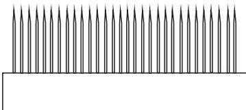
Make a board with holes to hold the required number of toothpicks. Drill the holes to the same depth as the holes in the sphere. Cut the toothpicks to length and place them, cut end in, in the board. Paint them white and while the paint is wet sprinkle glitter on them.
