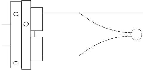
Take a piece of wood that is about 40mm square and 100mm long and mount it in a chuck. This length is needed so that a drill can reach all surfaces of the sphere. Or start with pin jaws and wood 20mm square but still 100mm long.
