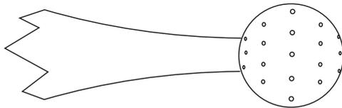
Drill holes all around the sphere. Measure your toothpicks and make these holes to fit. The star shown here has 36 holes. Every hole must point directly to the centre of the sphere. Part the sphere off. Put a dab of paint on the parting cut and sprinkle glitter on that paint.
