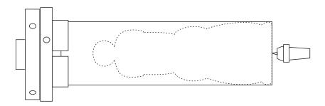
Turn to shape all except the very top of her hat. Sand all surfaces. If the wood is soft or porous give it a good coat of sanding sealer. Allow plenty of time to dry and sand again.
