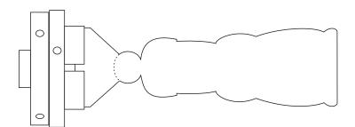
Part off and hand sand the top of the hat. Poke or drill a small hole in the top of the hat. Put the ends of a loop of string into this hole and glue them in. Or insert a small eyelet.
