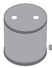
Add a connector for the hose from the vacuum pump. Regular compressed air fittings are recommended. Some vacuum tank plans show a vacuum gauge on the tank. If the operator can see into the tank a gauge is not needed. If a vacuum chuck pump is used as recommended above then that will have a vacuum gauge.
