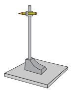
The centre height marker shown to us by Robbie Graham is used. For detailed drawings of this go to https://sawg.org.nz/tipsnjigs/ and select "Centre Height Marker".
