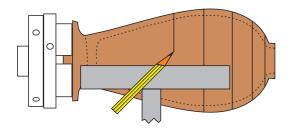
For simplicity the vertical lines are not shown here. You may draw either set of lines first. Decide on the spacing of the horizontal lines - these may be evenly spaced or closer at the top or bottom of the work. Bring a toolrest up to the work and draw the lines of your choice.
