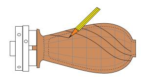
With both the horizontal and vertical lines on the work you can take a pencil and join the junction points of the lines to get repeated curves on the work for your decoration to follow.
