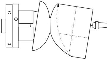
Mount in a chuck with the tailstock on one of the offset marks. Boldly mark the crossing point of the line down the side that extends from that offset. Make a vee cut as shown in the drawing. At the headstock end continue to cut until all the surface of the cylinder made earlier is gone. At the tailstock end continue to cut until you reach the mark at the crossing point of the lines. Sand both faces of the cut to a finished quality.
