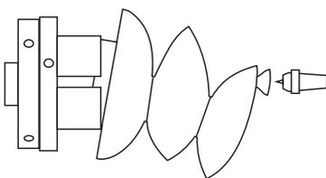
Remount the work in the chuck but this time with the tailstock up to the last of the offset marks. Make a vee cut as shown in the drawing. At the headstock end continue to cut until all the surface of the cylinder made earlier is gone. This will reduce the size of the disc on the headstock side of the cut. At the tailstock end cut until you have a knob suitable for lifting and shifting the tablet stand. Sand all surfaces to a finished quality.
