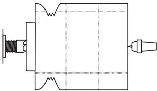
Mount the block between centres. Turn it to a cylinder and cut a 20 mm spigot to fit deep jaws on the bottom of the planned work. Extend the offset lines on the top down the sides of the cylinder. Draw lines around the cylinder at about thirds of the length. Start the cut to form the base of the stand.
