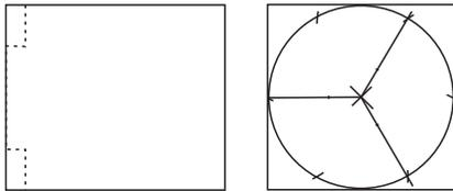
Mark a centre on each end. At the end that is to be the top draw a circle based on the centre mark. Keep the same compass setting and step around the circle to mark it into six equal parts. Draw a line from three of these marks to the centre. On each line mark a point 30 mm from the centre. Use an awl to mark each 30mm offset.
