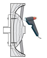
If you are planning thin legs at the corners of the work, or the wood is fragile, the corners will need some support. Apply a sealer to all of the underside of the work to reduce hot melt glue flow into the pores of the wood. Then use hot melt glue to add a wooden strut between each corner and the body of the work.
