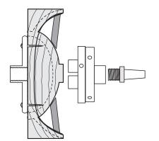
To get perfect consistency in the thickness of the square bowl edges and the size of the four feet it is very important to remount the bowl on a chuck perfectly. This can be helped by using a reverse adapter to hold a chuck on the tailstock. Slide the tailstock and chuck up to the bowl and grip the spigot. Now remove the entire assembly of faceplate, bowl, and chuck from the lathe. Remove the faceplate and return the work to the lathe mounted on the chuck.
