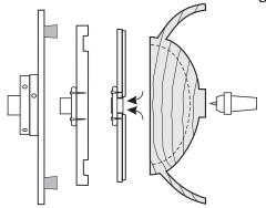
A square bowl of this shape may be held in Cole jaws (an external fit, possibly with shortened buttons), or a jam chuck, or a vacuum chuck, or pressed against a faceplate with the tailstock. It could have been designed with a taller bowl rim to ensure an easy fit in Cole jaws.
