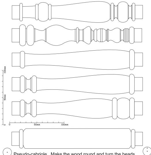
Pseudo-cabriole. Make the wood round and turn the beads. Then turn with each end off-centre while the other end is oncentre as shown below. The off-sets are on opposite sides. For a tapered cabriole cut the wood to a taper before shifting off-centre.
