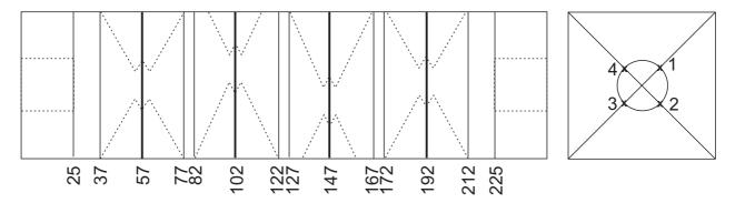
Start with a block 70 x 70 x 250mm long with the grain running lengthways. Mark the ends as above with four 12mm offsets. The numbers are the same on each end. Mount the wood between centres on the centre marks. Round the block and sand it. Make light and bold pencil marks as shown above. You may use a parting tool to cut a little way (just 2mm) down each bold line to show clearly where the cuts will be.
