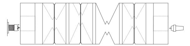
Remount the wood on one of the offset points. Cut one of the shapes close to the centre first. This may be done by starting with a parting tool down to a diameter of about 25mm and then completing the shape with spindle gouge and skew. Keep the sides of the cut at equal angles. Cut out to the light pencil marks. Sand all the cut area. When you understand the outcomes of the off-centre turning better you may cut beyond these lines on some cuts to produce a totally different look to the work.
