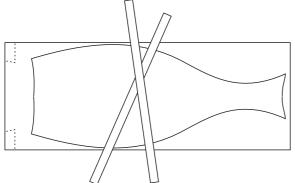
Cut the block. Make the faces perfectly flat. Glue in the laminate.
