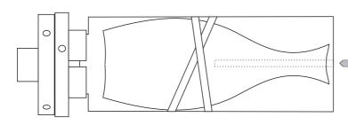
Mount the wood in a chuck. Round it off again. Drill the central hole then complete the top face of the vase.
