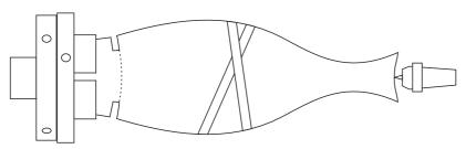
Bring up the tailstock to steady the wood.
