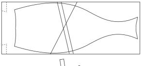
On the block of wood design the weed pot and the location of the laminations. If a second laminate is to cross the first then the cut width must be exactly the thickness of the laminate to be used.
