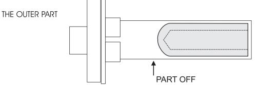
Mount one block in a scroll chuck and round it off. Dress the tailstock end and drill a 10 mm hole 40 mm into it. Measure this distance along the out edge of the drill bit so you get 40 mm of full width hole. Clean and finish the inside of this hole ensuring that the sides near the mouth remain perfectly parallel. Now thin the wood down to about 17 mm diameter. Part this off near the planned finished end and set it aside.
