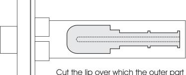
Cut the shaft down to 9 mm wide at the end and centre "wall" and 7 mm inbetween, where you will wind the cotton later.
