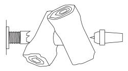
Glue the three pieces together so that the bits of branch wood are at 90° to each other and only a few millimetres of dowel is showing between them.
