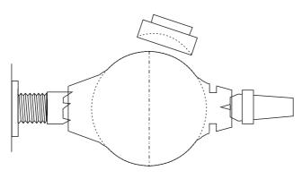
Turn it to a sort-of egg shape. Then proceed to make the centre portion exactly a part of a sphere to the left and right of the centre pencil line. Use the cup chuck, or any round object, to test for roundness. The edge of the measuring circle must be a perfect circle and when placed on the sphere there should be no gaps under this edge.
