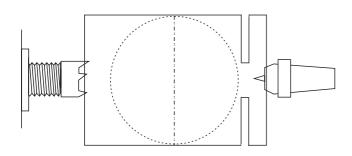
Mount a block between centres. This needs to be a little longer than it is wide. Round this off and mark a pencil line around the centre. If you wish you can measure the diameter and thus mark the left and right edges of the planned sphere. You can then cut outside this line with a parting tool.
