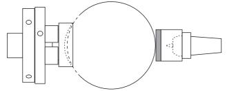
Sand and finish. This may require a few shifts of the wood between the cup chucks to enable sanding of the whole surface.
