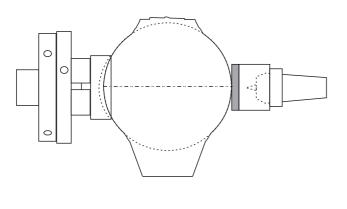
Re-mount the wood between the cup chuck and tail block. If you have made parting cuts then you can saw off the excess wood at this stage.
