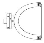
Turn the bowl over, hollow the inside, and cut the bowl rim to shape. Sand and finish the inside. Sand the resin further to 2000 grit. Then polish the resin with 3M Perfect-It 3000 Extra Cut Rubbing Compound, or one of the many other polishing compounds available.
