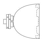
With the bowl mounted in a chuck cut a trench for the resin. Be sure that this is wide enough for the planned inserts. This trench needs to be a square cut, or a little wider at the bottom to ensure that the resin stays in place. Make the sides and bottom of the trench a nice smooth finish.
