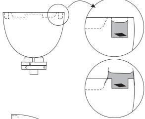
The depth of the trench, either as it is cut or with walls of masking tape added, must be enough for the poured resin to adequately cover all decorative inserts and allow for some of the resin to be cut away later to achieve a smooth finish.
