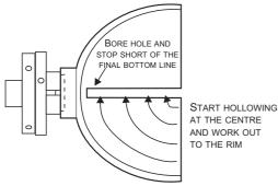
Re-mount the wood in a scroll chuck with the foot of the bowl towards the headstock. A hole drilled down the centre can make cutting easier and can be drilled to show you when you are nearing the required depth.
