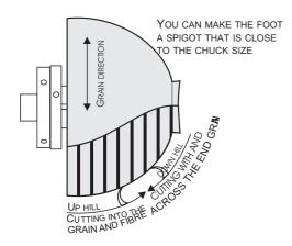
Mount the wood with the side that will become the top towards the headstock of the lathe. Use a faceplate, screw chuck or expand a scroll chuck into a drilled hole. Round the block off and make a dovetail recess or spigot for re-mounting. Shape the outside. Finishing cuts should be downhill for the best finish. You may choose to completely finish the outside at
