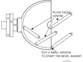
A hole drilled down the centre can make cutting easier and can be drilled to show you when you are nearing the required depth.
