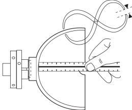
Check wall thickness and check the depth frequently as the bowl nears completion. Sand and finish the inside.
