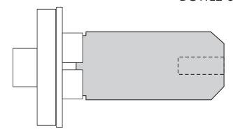
Mount a 85mm x 40mm x 40mm block by the corners in a 50mm chuck.
