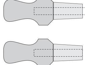
Glue a pre-drilled cork onto the dowel. Trim off the end of the dowel and sand that surface.
