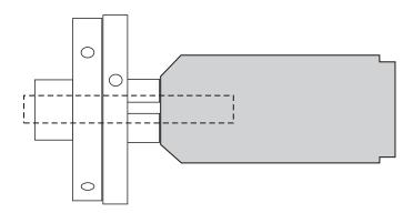
Glue a 55mm length of 10mm dowel into the hole. When the glue is set remount the piece in a small-jawed chuck.
